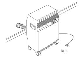
**Permanent installation** outlet holes must be in an exterior wall and opening diameter should not exceed 3"1/2.
